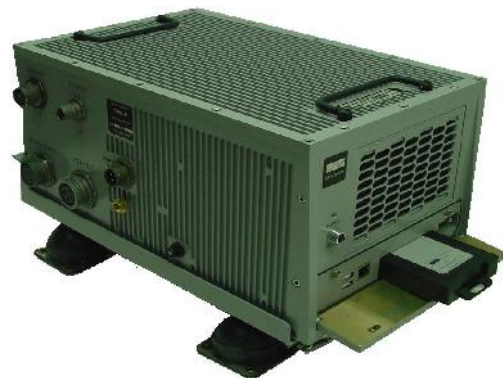
Standard shock mount Configuration
